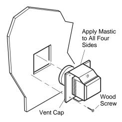
Figure 23 - Installing Horizontal Vent Cap
